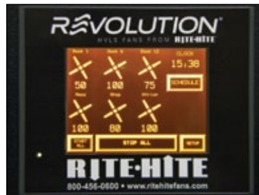
Rotating fan icons provide immediate visual of fan operation
