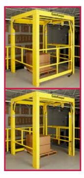
When the outer gate opens to allow pallets to enter the mezzanine, the inner gate automatically closes to keep workers out. After the pallet is received, mezzanine-level workers open the inner gate to remove material from the work zone while the outer gate closes to secure the leading edge of the platform. To prevent the outer gate from being raised by a worker inside the work zone, a Saf-T-Latch is integrated that can only be accessed when standing outside the work zone.
