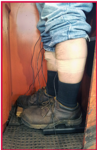
An accelerometer affixed to a fork lift operator's lower leg measures tibial shock.
