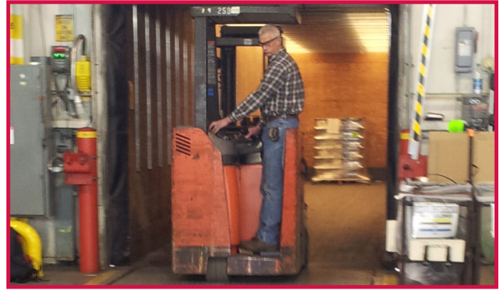
A forklift operator exits a semi-trailer during a “dock shock” study conducted by The Ohio State University.
