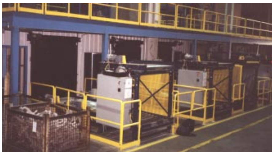
Four Guardian Barrier Curtains from Frommelt Safety Products help to minimize the time required for castings to enter the inspection room, maintaining the darkroom environment and improving plant efficiency.
