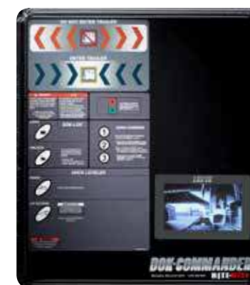
A single Dok-Commander system offers simple access to controls for each dock component.
