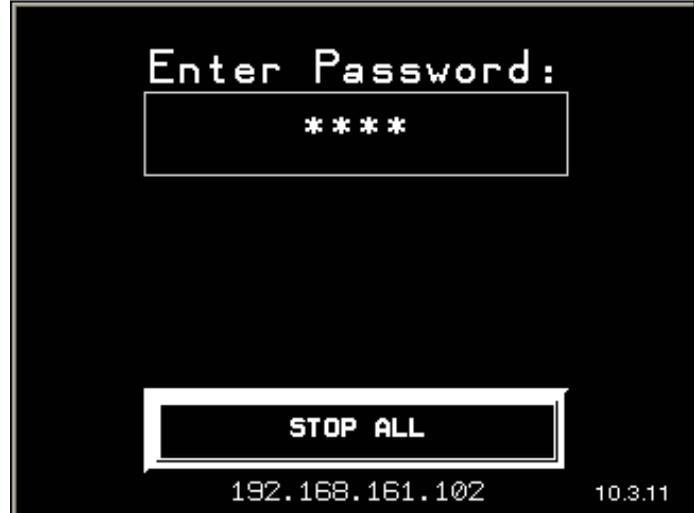
Set Password allows the user to define a custom password to access the Fan-Commander. Touch the box to enter the new password.
