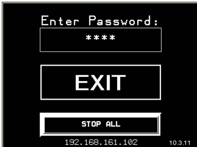
In the center of the **LOGIN** screen is an **EXIT** button. This allows unauthorized users to return to the **ZONE CONTROL** screen.
