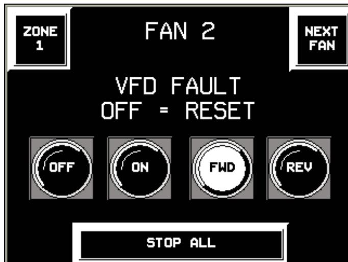
Verify that there are no visible causes for the fault (ie obstruction or impact) before resetting a fault.
